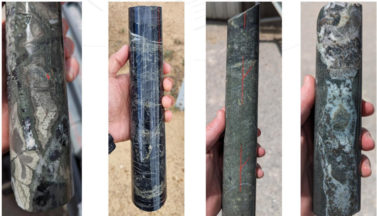
Figure 5: Selection of drill core from the three deep drill holes displaying alteration and mineralisation at depth.
