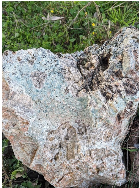
Figure 8: green, glassy auto brecciated rhyolite (sample 71668).
