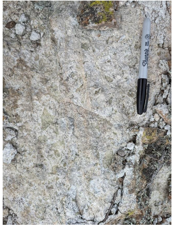
Figure 7: strongly clay altered pyroclastic volcanic (sample 72432).
